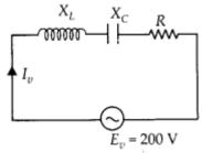
Average power transferred to the circuit in one complete cycle at resonance  $P = E_n I_n \cos \phi$
