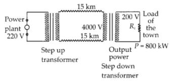
Line resistance = length of two wire line × resistance per unit length
