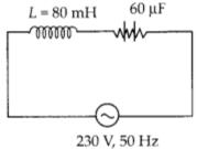
(a) Inductive reactance ,  $X_L = 2\pi f L$  $X_L = 2\pi (50) \ 80 \times 10^{-3} = 25.12 \ \Omega$
